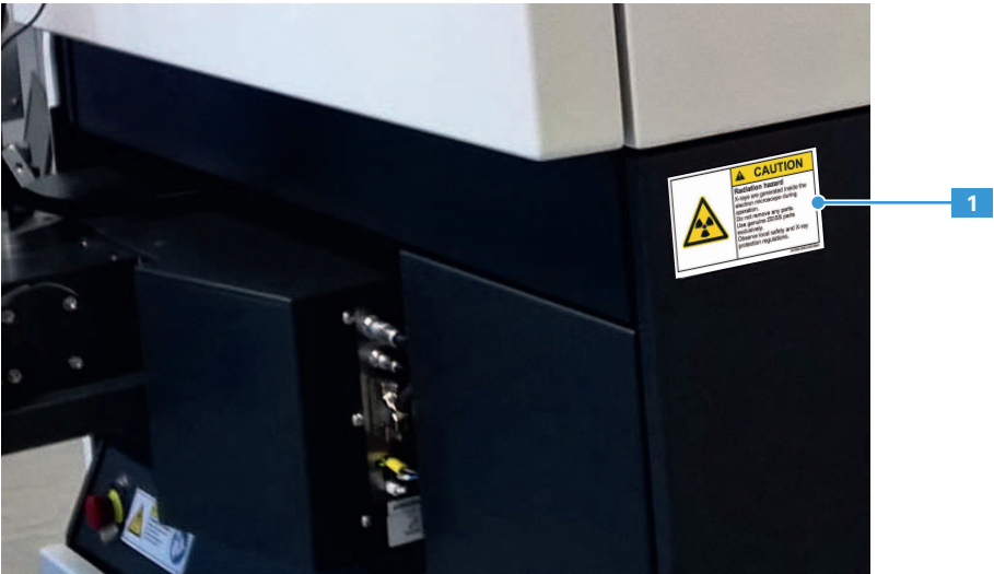
Fig. 2.7: Safety label on the back side of the microscope cabinet
