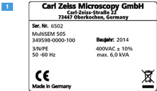
Fig. 2.9: Safety label and type plate at the bottom of the power supply rack
