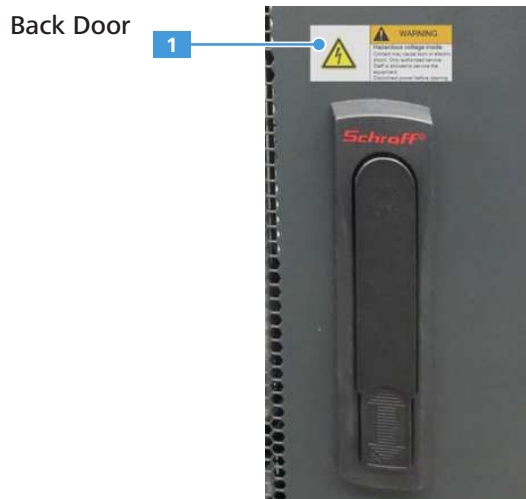
Fig. 2.12: Safety label at the back door of the image acquisition rack
