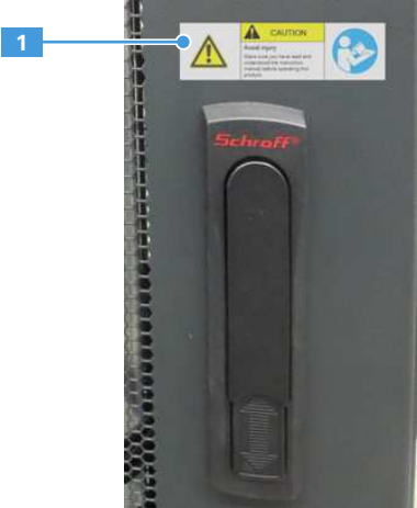
Fig. 2.11: Safety label at the front door of the image acquisition rack
