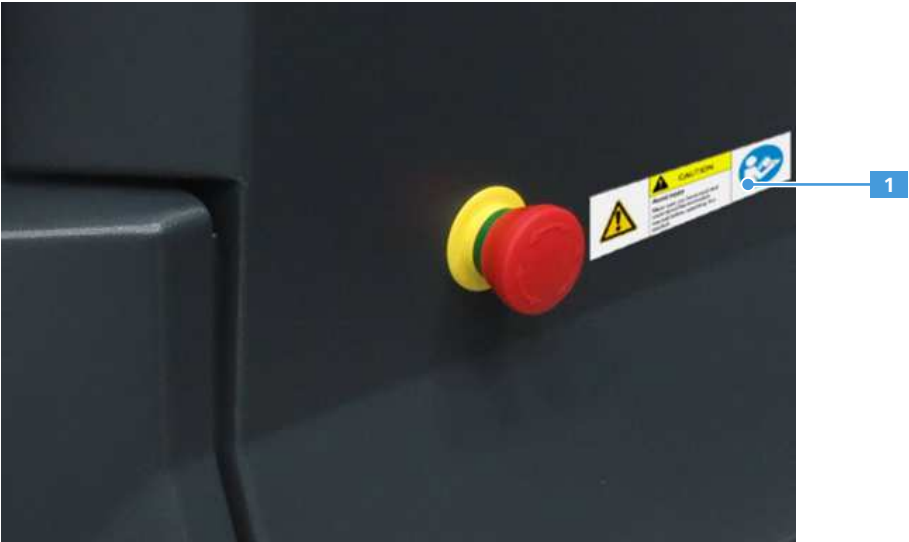
Fig. 2.6: Safety label on the right side of the microscope cabinet
