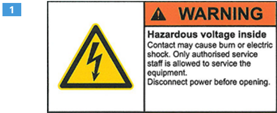
Fig. 2.10: Safety label at the back door of the power supply rack
