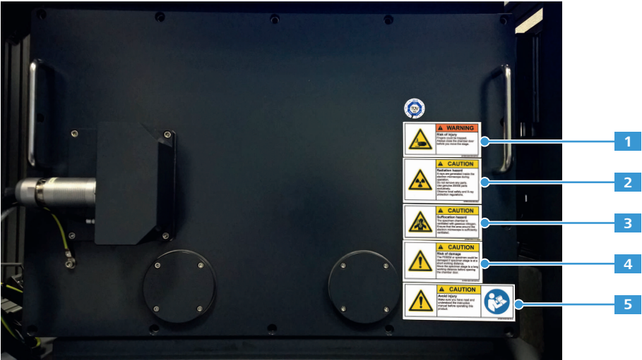
Fig. 2.5: Safety labels on the chamber door
