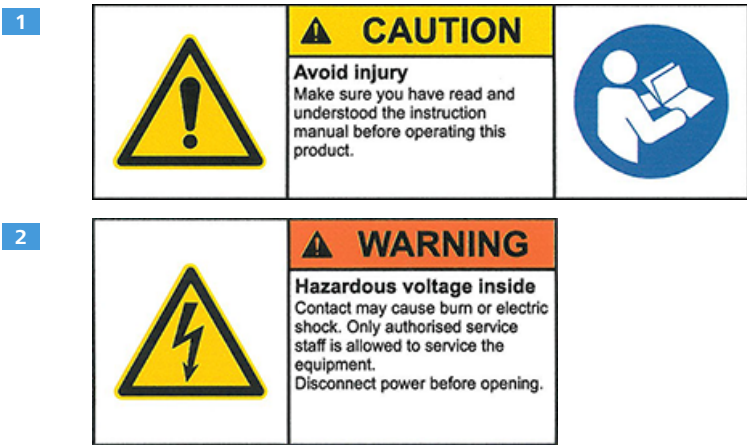
Fig. 2.8: Safety labels at the main switch area
